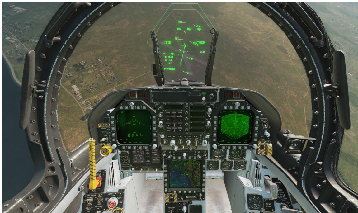
Figure 9. Rolling out on the Aim Off Point (slightly steep but within parameters). Note it is above the target. The AoA is around 1, as expected.
