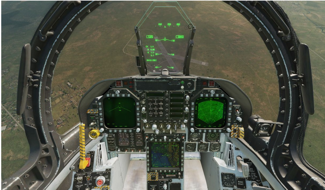
Figure 10. The moment of weapon release, when the CCIP flashes off. Note the parameters of 535KCAS and 3800ft. This is a valid release.
