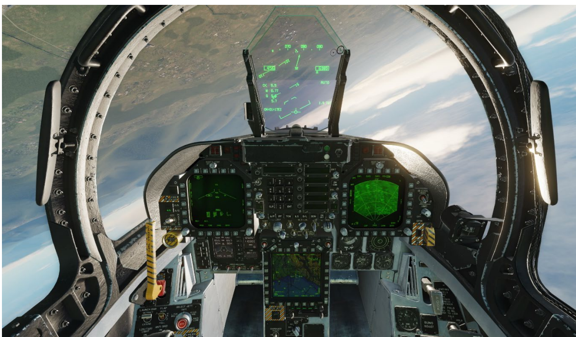
Figure 7. Rolling in. Using 5+ g the altitude peaks out at ~7000ft above target altitude.
