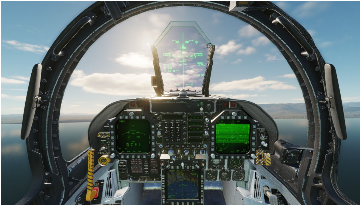
Figure 3. In the 3g pull up, note the VV has just passed the dive bars.
