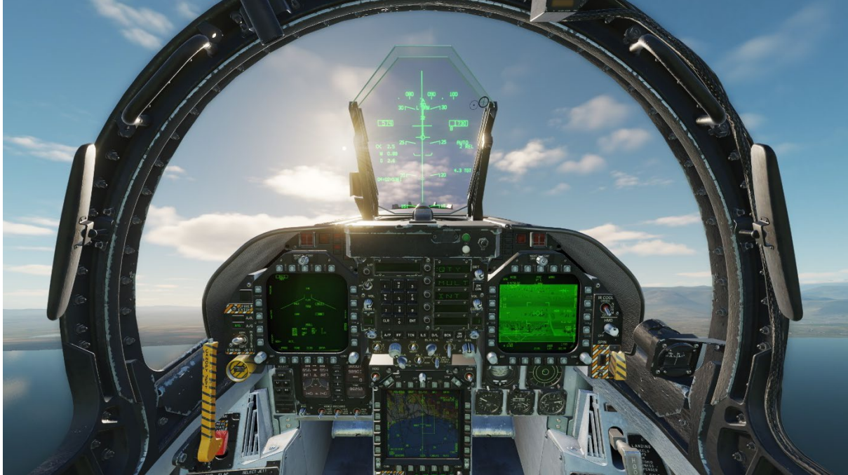
Figure 4. On the ASL, with the release cue about to hit the VV.
